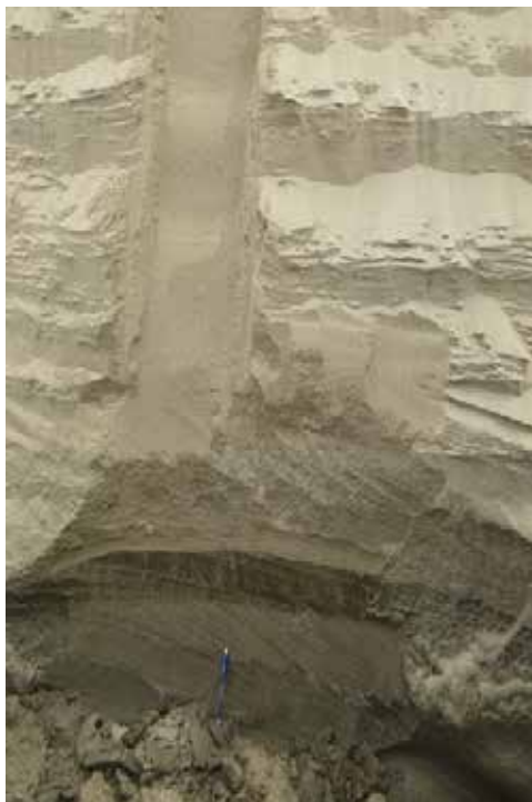
Figure 14: Channel sample and dark grey cross bedded heavy mineral rich layer (above the pencil) ~6cm thick at ECS-02
