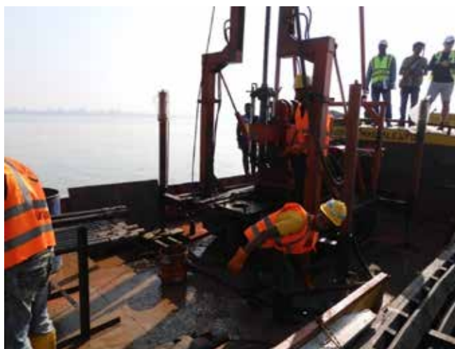
Figure 17: Drilling set up on customised river vessel for sampling in active channel.
